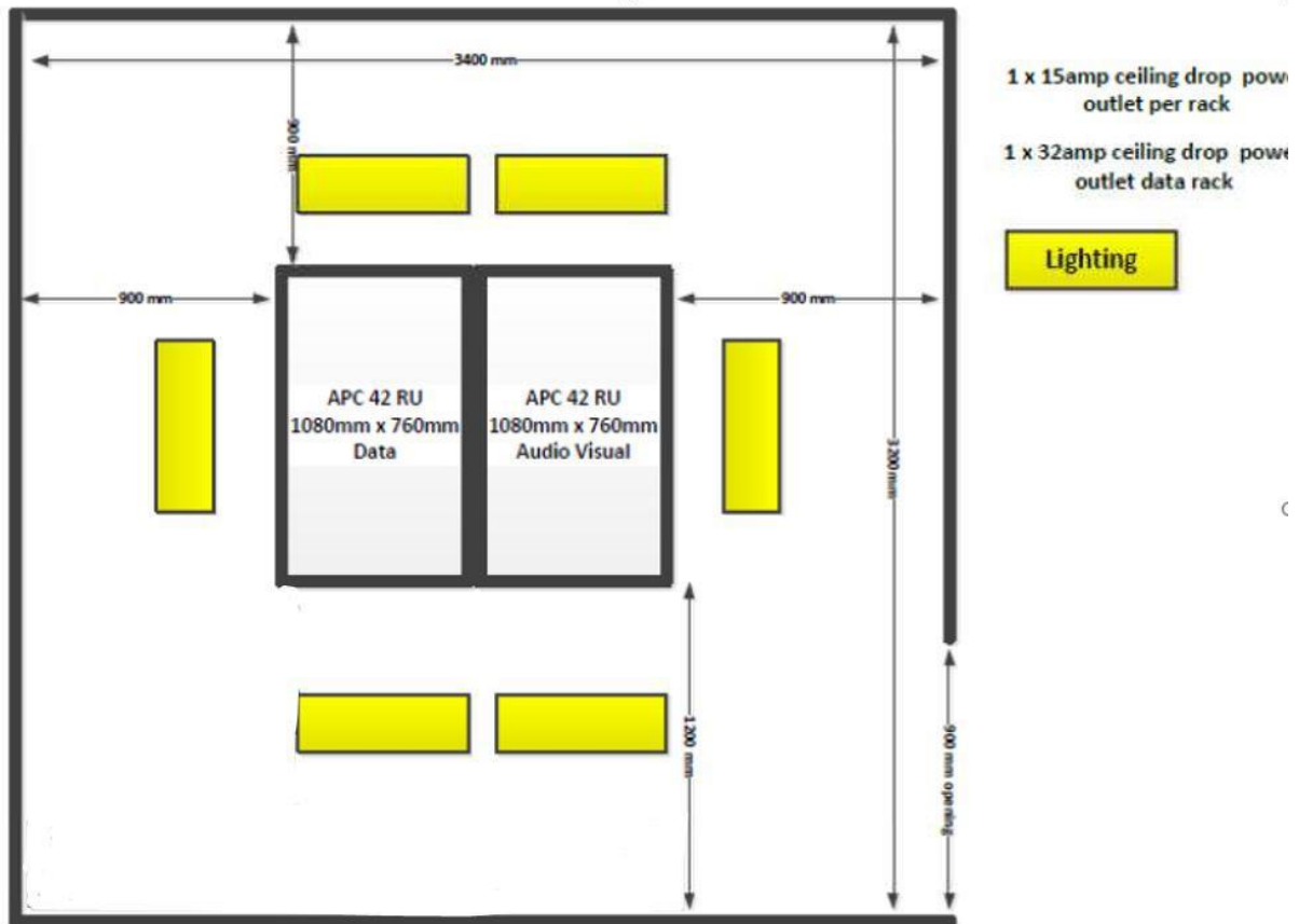
Standard 2 rack communications room
